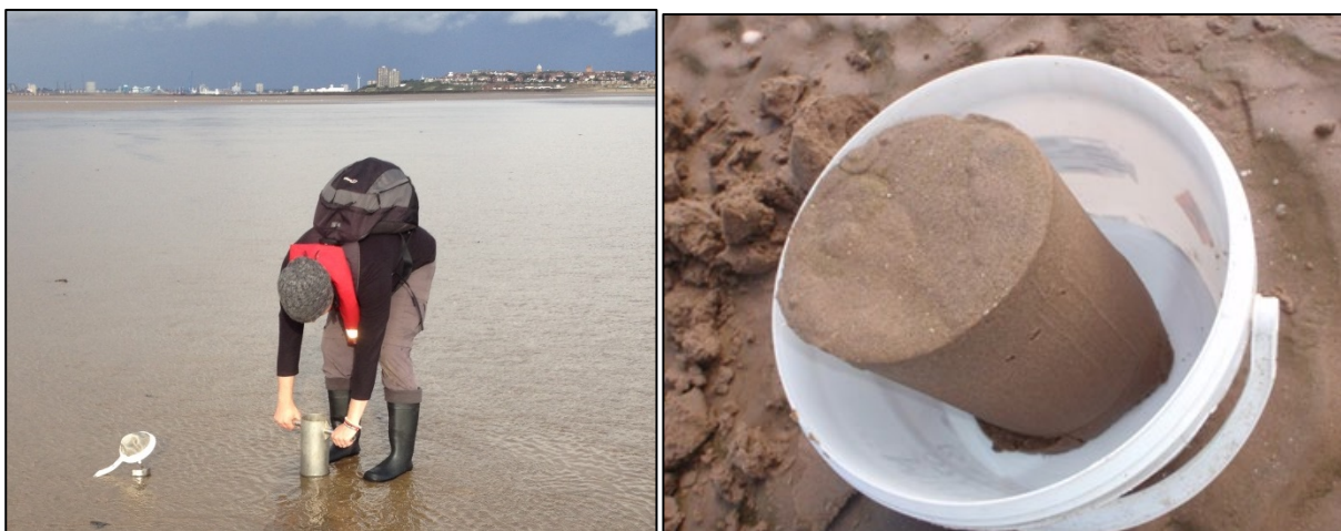
Figure 3. Deploying a hand corer (left) and a sediment core after collection (right) Images © APEM Ltd
