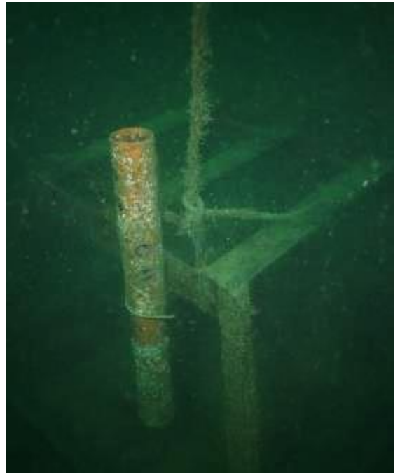
Passive sediment trap on seabed at Skomer MCZ
